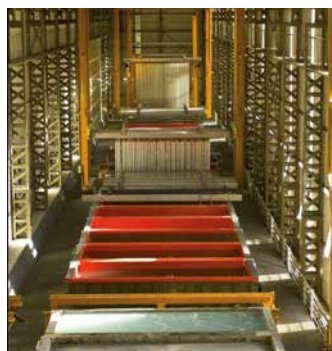
Fully automated vertical anodising plant for architectural profiles with online additional powder coating facilities.
